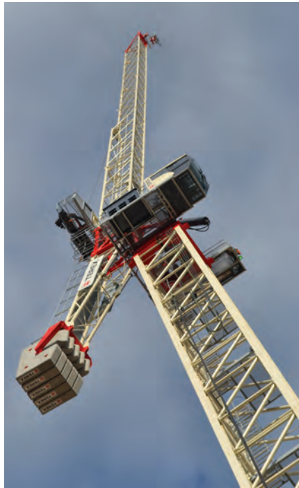
LEFT AND RIGHT: The Terex CTLH 192-12 hydraulic luffing jib tower crane offers a maximum capacity of 12 t, with a jib of up to 55 m and a tip load of up to 2.35 t
