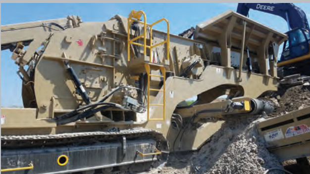
ABOVE AND RIGHT: Kolberg-Pioneer has added a two-deck, 4-ft x 7-ft pre-screen option to its FT4250 mobile impactor plant.
