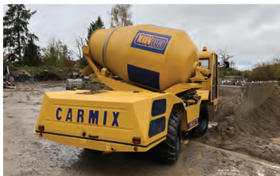
ALL IMAGES: Garten Richter has selected a Carmix 3.5 TT mobile concrete batching plant to help build concrete blocks (measuring 180 x 60 x 60 cm) in the shape of Lego bricks with recycled material.
