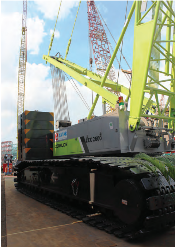
The Zoomlion ZCC2600 crawler crane has an operating weight of about 220 t and a maximum boom length of 83 m. Its fixed jib is 12-30 m long, while the luffing jib is up to 60 m long.
