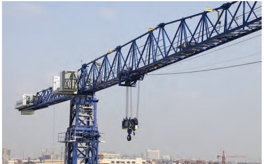
ABOVE AND LEFT: The new Comansa 21CM750 flat-top crane offers two maximum capacities, 37.5 t and 50 t. It is targeted at the Asian market, but will also be distributed in South America, the Middle East and Africa.
