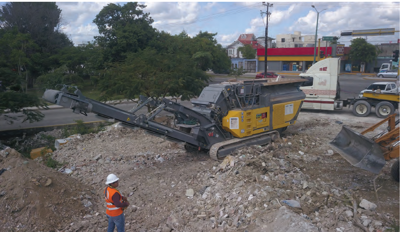
TOP AND ABOVE: The RM 100GO! mobile crusher from Rubble Master working in the Mexican city of Cancún to transform construction and demolition waste into valuable final materials. These recycled materials are then used directly on site for fillings and the substructure of roads.
