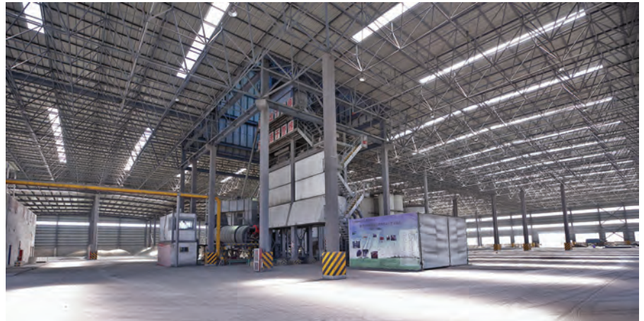
ABOVE AND LEFT: The Ammann ABA 320 UniBatch asphalt plant (above), located inside a factory, is working on a new district development in China. The unit is expected to operate almost continuously over the next decade.
