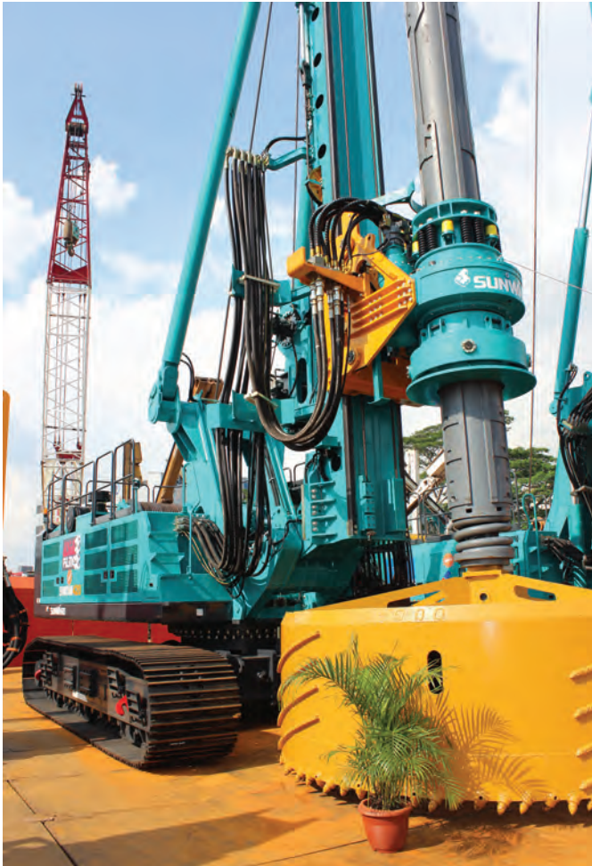
ABOVE AND BELOW: The Sunward SWDM420 has a maximum torque of 420 kN, drilling diameter of 2,800 mm and drilling depth of 110 m.
