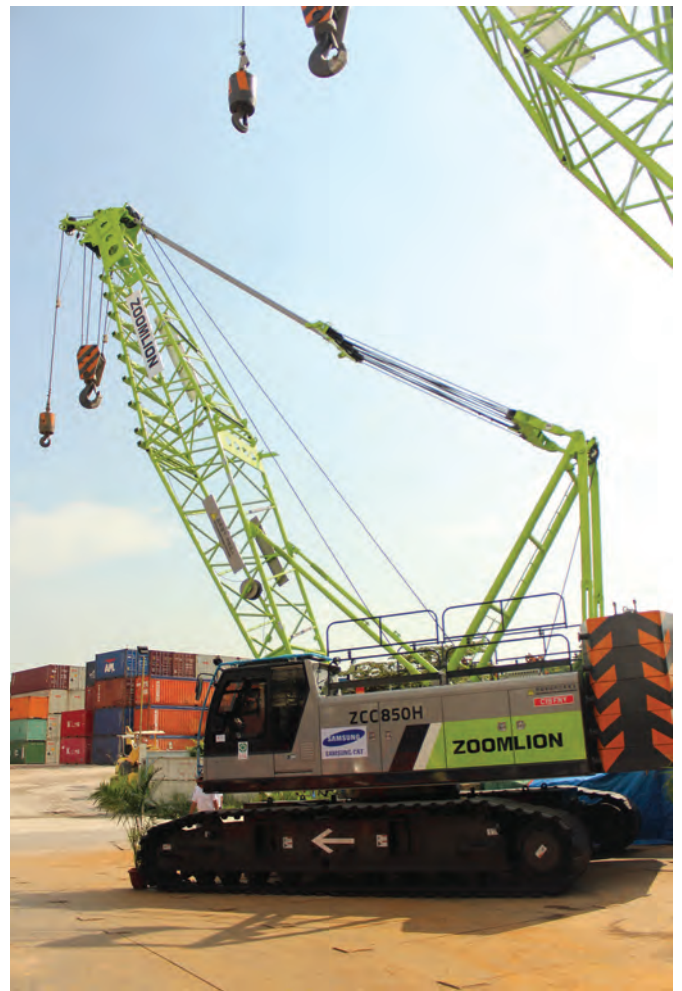
ABOVE AND RIGHT: The Zoomlion ZCC850H offers a boom length of 13 – 61 m, fixed jib length of 7 – 19 m and maximum lifting moment of 357 tm.
