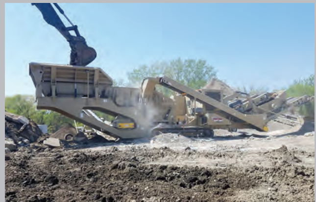
ABOVE AND RIGHT: Kolberg-Pioneer has added a two-deck, 4-ft x 7-ft pre-screen option to its FT4250 mobile impactor plant.
