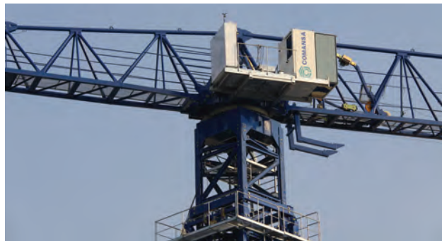
ABOVE AND LEFT: The new Comansa 21CM750 flat-top crane offers two maximum capacities, 37.5 t and 50 t. It is targeted at the Asian market, but will also be distributed in South America, the Middle East and Africa.
