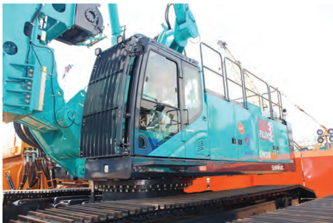
ABOVE AND BELOW: The Sunward SWDM420 has a maximum torque of 420 kN, drilling diameter of 2,800 mm and drilling depth of 110 m.
