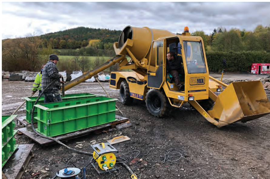
ALL IMAGES: Garten Richter has selected a Carmix 3.5 TT mobile concrete batching plant to help build concrete blocks (measuring 180 x 60 x 60 cm) in the shape of Lego bricks with recycled material.
