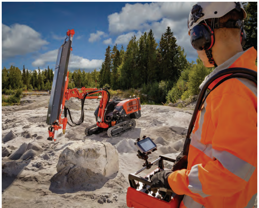
TOP AND ABOVE: The new Dino DC410Ri surface top hammer drill rig is designed for 51- to 76-mm hole sizes. It offers mobility and stability for contractors tackling cramped urban construction sites, as well as for demanding quarry and infrastructure applications.
