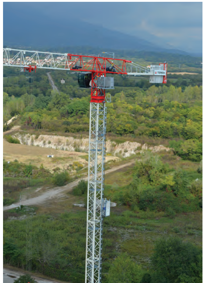
RIGHT: The CTT 172-8 is the latest flat-top tower crane from Terex with a maximum capacity of 8 t and a jib reaching 65 m length. The load capacity at maximum length is up to 1.71 t.
