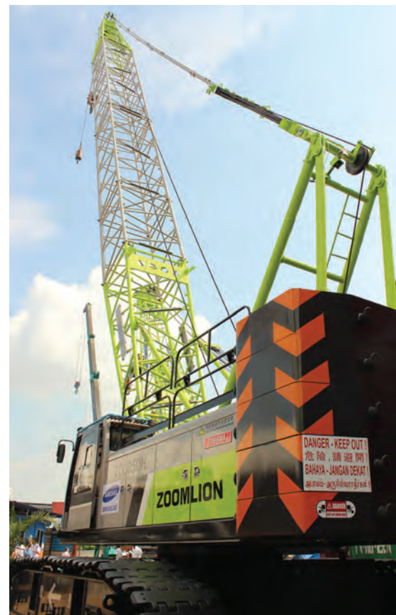
ABOVE AND RIGHT: The Zoomlion ZCC850H offers a boom length of 13 – 61 m, fixed jib length of 7 – 19 m and maximum lifting moment of 357 tm.
